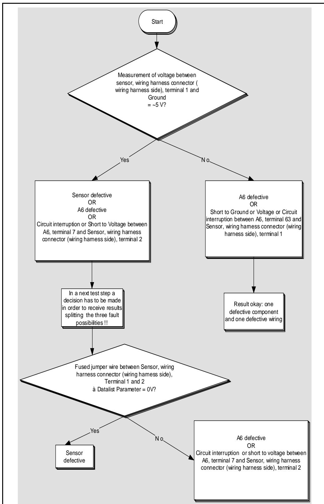
**Figure 42** Engine Coolant Temperature FIP@GM
