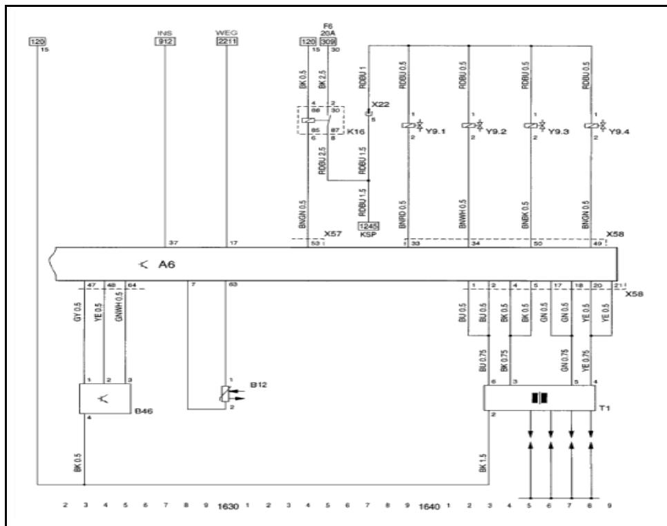
Figure 40 Wiring schematic diagram example@GM
