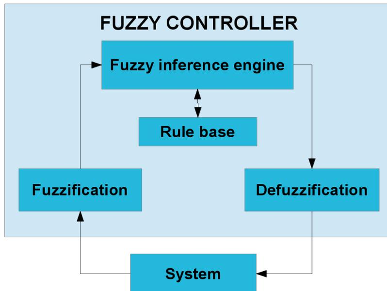
**Fig. 3.** Block diagram of a fuzzy controller
