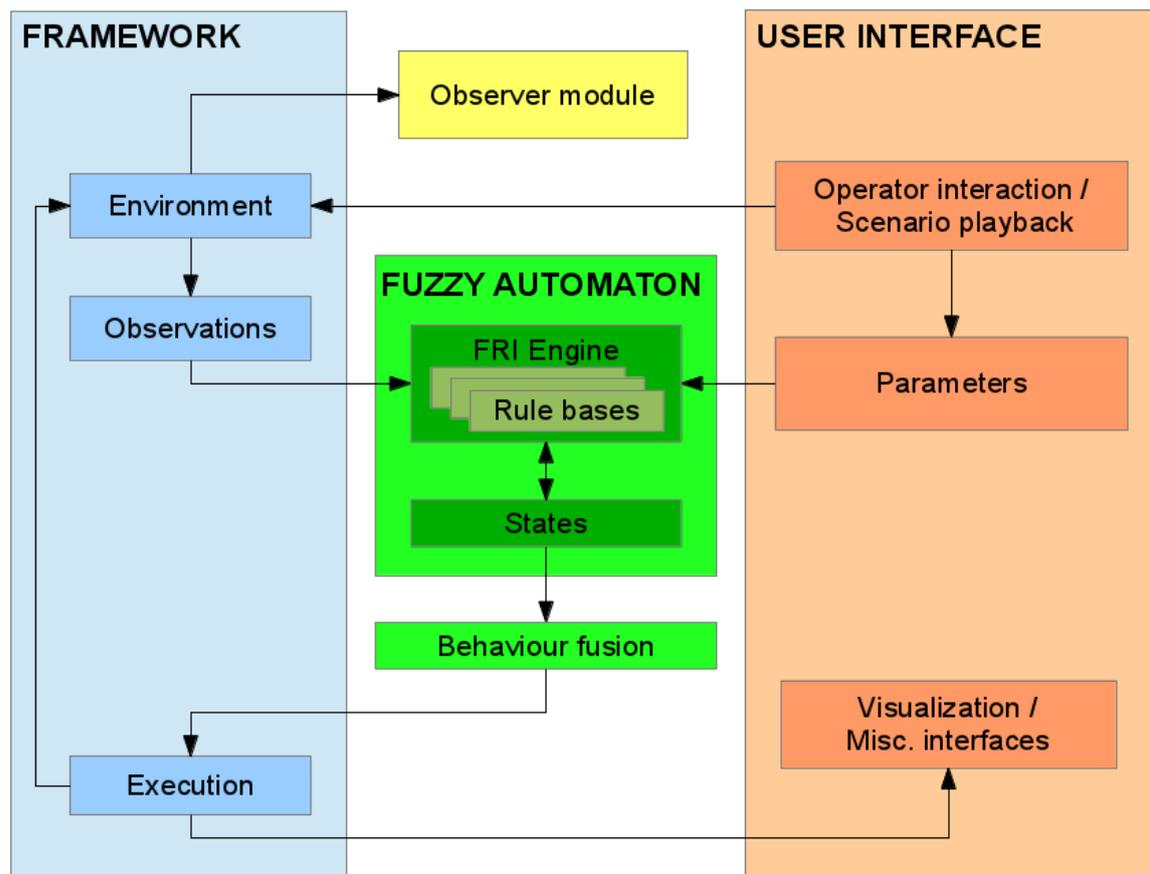
**Fig. 28.** Structure of the simulation implementation
