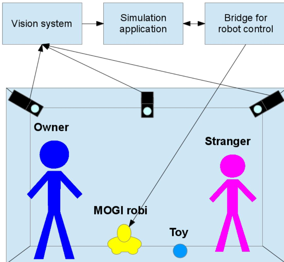
**Fig. 38.** Schematic diagram of the ‘MOGI robi’ in Intelligent Space
