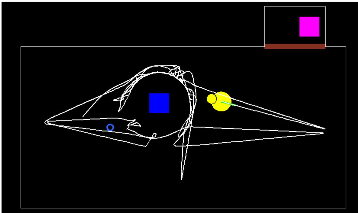
Fig. 30. A sample track induced by the exploration behaviour component
